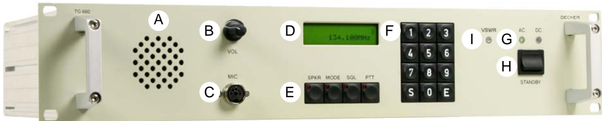
Figure 15: TG660 – Controls and Indications
